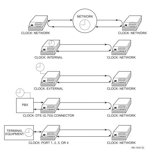
Figure 3-12. Common Clocking Configurations
